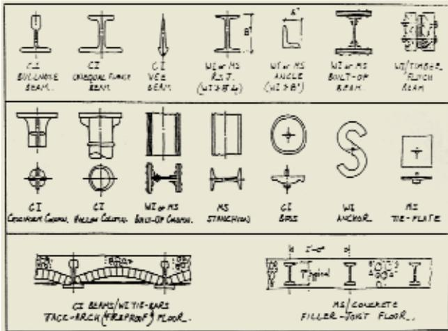
Common structural forms. C.I.= cast iron. W.I.= wrought iron M.S.= mild steel
