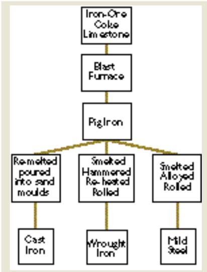
Flow chart of the manufacture of metalwork
